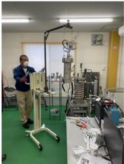
Slide-1: NHFE Reactor No.1; setting reactor chamber into outer thermal isolation chamber with water cooling coil on surface. Currently several reactors are running for accumulating R&D data.
